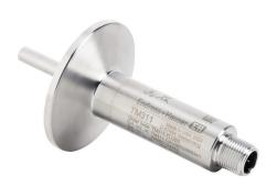
Endress+Hauser iTHERM temperature sensor/transmitter, Pt100 RTD, M12 probe, 0 to 150 deg C, 30mm insertion length, 6mm probe diameter, 1-1/2in sanitary tri-clamp process connection, Output: 1-channel, current/IO-Link, 4-pin M12 quick-disconnect.
