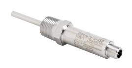
Endress+Hauser iTHERM temperature sensor/transmitter, Pt100 RTD, M12 probe, 0 to 150 deg C, 50mm insertion length, 6mm probe diameter, 1/2in male NPT process connection, Output: 1-channel, current/IO-Link, 4-pin M12 quick-disconnect.
