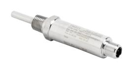
Endress+Hauser iTHERM temperature sensor/transmitter, Pt100 RTD, M12 probe, 0 to 150 deg C, 30mm insertion length, 6mm probe diameter, 1/4in male NPT process connection, Output: 1-channel, current/IO-Link, 4-pin M12 quick-disconnect.
