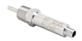
Endress+Hauser iTHERM temperature sensor/transmitter, Pt100 RTD, M12 probe, 0 to 150 deg C, 30mm insertion length, 6mm probe diameter, 1/2in male NPT process connection, Output: 1-channel, current/IO-Link, 4-pin M12 quick-disconnect.
