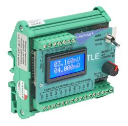
Laumas analog load cell transmitter, (4) load cell input(s), +/-39 mV, analog output, Modbus RTU, 12-24 VDC operating voltage. For use with 4- or 6-wire load cells. Up to (8) load cells can be connected.
