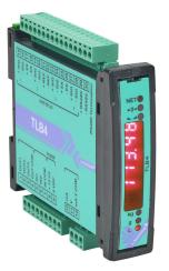
Laumas discrete/analog load cell transmitter, (4) load cell input(s), +/- 39 mV, analog and relay output, Modbus RTU, 12-24 VDC operating voltage. For use with 4- or 6-wire load cells. Up to (16) load cells can be connected.
