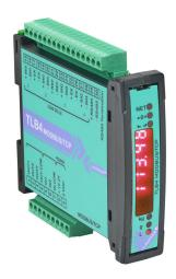
Laumas discrete load cell transmitter, (4) load cell input(s), +/-39 mV, relay output, Modbus RTU and Modbus TCP, 12-24 VDC operating voltage. For use with 4- or 6-wire load cells. Up to (16) load cells can be connected.
