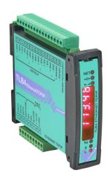
Laumas discrete load cell transmitter, (4) load cell input(s), +/-39 mV, relay output, Modbus RTU and webserver, 12-24 VDC operating voltage. For use with 4- or 6-wire load cells. Up to (16) load cells can be connected.
