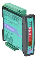
Laumas discrete load cell transmitter, (4) load cell input(s), +/-39 mV, relay output, EtherNet/IP and Modbus RTU, 12-24 VDC operating voltage. For use with 4- or 6-wire load cells. Up to (16) load cells can be connected.
