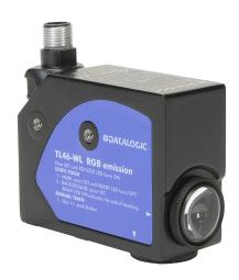
Datalogic contrast sensor, rectangular, diffuse, RGB, horizontal spot orientation, 6-12mm sensing distance, selectable light-on/dark-on, NPN/PNP, teach-in button, 20 kHz switching frequency, aluminum housing, 5-pin M12 quick-disconnect.
