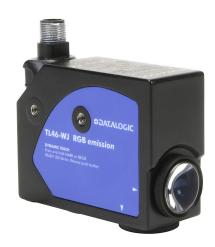
Datalogic contrast sensor, rectangular, diffuse, RGB light emission, vertical spot orientation, 6-12mm sensing distance, selectable light-on/dark-on, PNP, teach-in button, 50 kHz switching frequency, aluminum housing, 5-pin M12 quick-disconnect.
