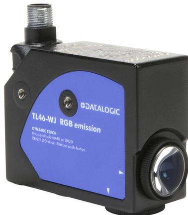
Datalogic contrast sensor, rectangular, diffuse, RGB, vertical spot orientation, 6-12mm sensing distance, selectable light-on/dark-on, PNP, teach-in button, 50 kHz switching frequency, aluminum housing, 5-pin M12 quick-disconnect.
