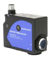
Datalogic contrast sensor, rectangular, diffuse, RGB, horizontal spot orientation, 6-12mm sensing distance, selectable light-on/dark-on, PNP, teach-in button, 50 kHz switching frequency, aluminum housing, 5-pin M12 quick-disconnect.
