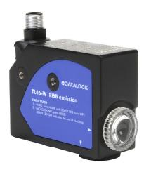
Datalogic contrast sensor, rectangular, diffuse, RGB light emission, vertical spot orientation, 6-12mm sensing distance, selectable light-on/dark-on, NPN/PNP, teach-in button, 15 kHz switching frequency, aluminum housing, 5-pin M12 quickdisconnect.
