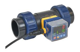
ICON Process Controls Truflo flow meter, paddle wheel, 1-1/2in schedule 80 PVC socket process connection, 6.5 to 225 GPM, 0 to 999,999 gallons, Output 1: switch, Output 2: switch or pulse, Output 3: analog.
