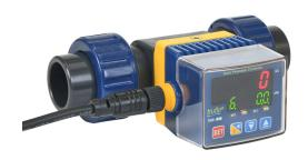
ICON Process Controls Truflo flow meter, paddle wheel, 3/4in schedule 80 PVC socket process connection, 1.5 to 45 GPM, 0 to 999,999 gallons, Output 1: switch, Output 2: switch or pulse, Output 3: analog.
