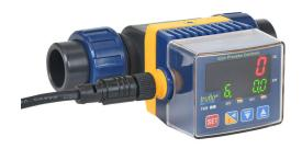
ICON Process Controls Truflo flow meter, paddle wheel, 1/2in schedule 80 PVC socket process connection, 1 to 32 GPM, 0 to 999,999 gallons, Output 1: switch, Output 2: switch or pulse, Output 3: analog.
