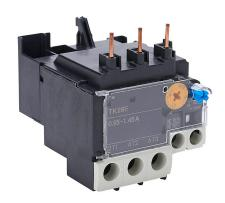
Fuji Electric TK26E series thermal overload relay, 0.95-1.45A adjustable, bi-metallic, direct mount power connection(s). For use with SC-E02x, SC-E03x, SC-E04x and SC-E05x contactors.
