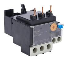
Fuji Electric TK26E series thermal overload relay, 0.8-1.2A adjustable, bi-metallic, direct mount power connection(s). For use with SC-E02x, SC-E03x, SC-E04x and SC-E05x contactors.
