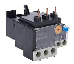
Fuji Electric TK26E series thermal overload relay, 0.64-0.96A adjustable, bi-metallic, direct mount power connection(s). For use with SC-E02x, SC-E03x, SC-E04x and SC-E05x contactors.
