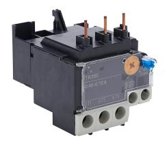
Fuji Electric TK26E series thermal overload relay, 0.48-0.72A adjustable, bi-metallic, direct mount power connection(s). For use with SC-E02x, SC-E03x, SC-E04x and SC-E05x contactors.
