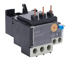
Fuji Electric TK26E series thermal overload relay, 0.18-0.27A adjustable, bi-metallic, direct mount power connection(s). For use with SC-E02x, SC-E03x, SC-E04x and SC-E05x contactors.
