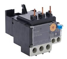
Fuji Electric TK26E series thermal overload relay, 0.13-0.20A adjustable, bi-metallic, direct mount power connection(s). For use with SC-E02x, SC-E03x, SC-E04x and SC-E05x contactors.
