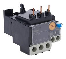
Fuji Electric TK26E series thermal overload relay, 1.4-2.1A adjustable, bi-metallic, direct mount power connection(s). For use with SC-E02x, SC-E03x, SC-E04x and SC-E05x contactors.
