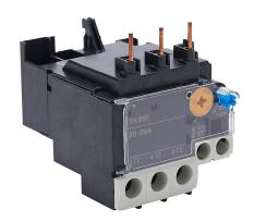
Fuji Electric TK26E series thermal overload relay, 20.0-26.0A adjustable, bi-metallic, direct mount power connection(s). For use with SC-E05x contactors.
