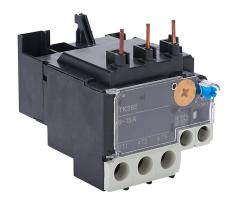
Fuji Electric TK26E series thermal overload relay, 9.0-13.0A adjustable, bi-metallic, direct mount power connection(s). For use with SC-E03x, SC-E04x and SC-E05x contactors.
