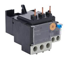
Fuji Electric TK26E series thermal overload relay, 7.0-10.5A adjustable, bi-metallic, direct mount power connection(s). For use with SC-E02x, SC-E03x, SC-E04x and SC-E05x contactors.
