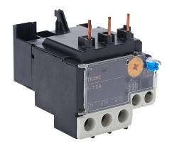
Fuji Electric TK26E series thermal overload relay, 5.0-7.5A adjustable, bi-metallic, direct mount power connection(s). For use with SC-E02x, SC-E03x, SC-E04x and SC-E05x contactors.
