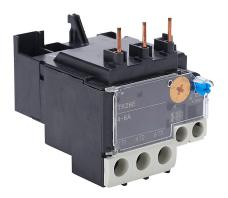
Fuji Electric TK26E series thermal overload relay, 4.0-6.0A adjustable, bi-metallic, direct mount power connection(s). For use with SC-E02x, SC-E03x, SC-E04x and SC-E05x contactors.
