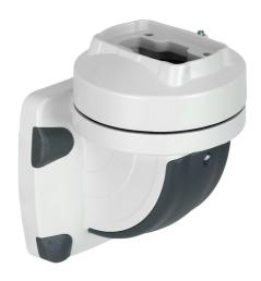
Teknokol suspension arm fitting, right-angle wall-mount swivel base, 310 degrees movement range, aluminum, RAL 7035 light gray. For use with TK060 suspension arm profile.
