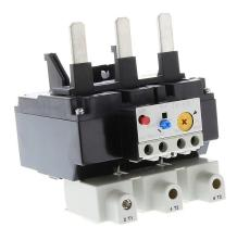
Fuji Electric TK-E6 series thermal overload relay, 53.0-80.0A adjustable, bi-metallic, direct mount power connection(s). For use with SC-E6x and SC-E7x contactors.
