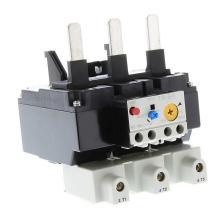
Fuji Electric TK-E6 series thermal overload relay, 85.0-125.0A adjustable, bi-metallic, direct mount power connection(s). For use with SC-E6x and SC-E7x contactors.
