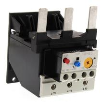
Fuji Electric TK-E5 series thermal overload relay, 65.0-95.0A adjustable, bi-metallic, direct mount power connection(s), panel mount. For use with SC-E5x contactors.
