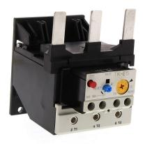
Fuji Electric TK-E5 series thermal overload relay, 45.0-65.0A adjustable, bi-metallic, direct mount power connection(s), panel mount. For use with SC-E5x contactors.
