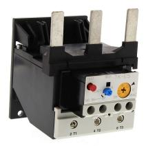
Fuji Electric TK-E5 series thermal overload relay, 34.0-50.0A adjustable, bi-metallic, direct mount power connection(s), panel mount. For use with SC-E5x contactors.
