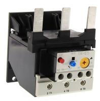
Fuji Electric TK-E5 series thermal overload relay, 85.0-105.0A adjustable, bi-metallic, direct mount power connection(s), panel mount. For use with SC-E5x contactors.
