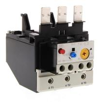
Fuji Electric TK-E3 series thermal overload relay, 64.0-80.0A adjustable, bi-metallic, direct mount power connection(s). For use with SC-E4x contactors.
