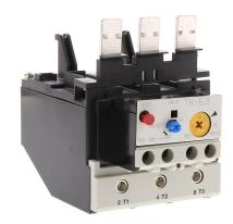
Fuji Electric TK-E3 series thermal overload relay, 48.0-68.0A adjustable, bi-metallic, direct mount power connection(s). For use with SC-E3x and SC-E4x contactors.
