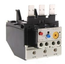
Fuji Electric TK-E3 series thermal overload relay, 45.0-65.0A adjustable, bi-metallic, direct mount power connection(s). For use with SC-E3x and SC-E4x contactors.
