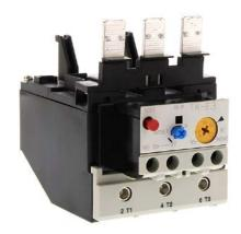
Fuji Electric TK-E3 series thermal overload relay, 34.0-50.0A adjustable, bi-metallic, direct mount power connection(s). For use with SC-E3x and SC-E4x contactors.
