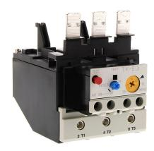
Fuji Electric TK-E3 series thermal overload relay, 34.0-50.0A adjustable, bi-metallic, direct mount power connection(s). For use with SC-E3x and SC-E4x contactors.
