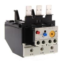
Fuji Electric TK-E3 series thermal overload relay, 28.0-40.0A adjustable, bi-metallic, direct mount power connection(s). For use with SC-E3x and SC-E4x contactors.
