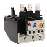
Fuji Electric TK-E3 series thermal overload relay, 24.0-36.0A adjustable, bi-metallic, direct mount power connection(s). For use with SC-E3x and SC-E4x contactors.
