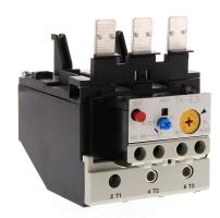
Fuji Electric TK-E3 series thermal overload relay, 18.0-26.0A adjustable, bi-metallic, direct mount power connection(s). For use with SC-E3x and SC-E4x contactors.
