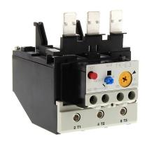
Fuji Electric TK-E3 series thermal overload relay, 12.0-18.0A adjustable, bi-metallic, direct mount power connection(s). For use with SC-E3x and SC-E4x contactors.
