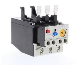
Fuji Electric TK-E2 series thermal overload relay, 5.0-8.0A adjustable, bi-metallic, direct mount power connection(s). For use with SC-E1x, SC-E2x and SC-E2Sx contactors.
