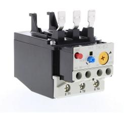
Fuji Electric TK-E2 series thermal overload relay, 44.0-54.0A adjustable, bi-metallic, direct mount power connection(s). For use with SC-E1x, SC-E2x and SC-E2Sx contactors.
