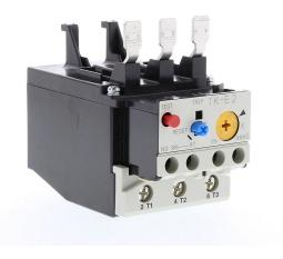
Fuji Electric TK-E2 series thermal overload relay, 40.0-50.0A adjustable, bi-metallic, direct mount power connection(s). For use with SC-E1x, SC-E2x and SC-E2Sx contactors.
