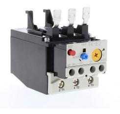
Fuji Electric TK-E2 series thermal overload relay, 24.0-36.0A adjustable, bi-metallic, direct mount power connection(s). For use with SC-E1x, SC-E2x and SC-E2Sx contactors.
