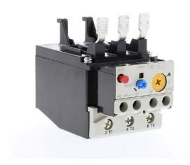
Fuji Electric TK-E2 series thermal overload relay, 24.0-36.0A adjustable, bi-metallic, direct mount power connection(s). For use with SC-E1x, SC-E2x and SC-E2Sx contactors.
