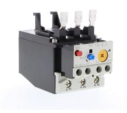
Fuji Electric TK-E2 series thermal overload relay, 18.0-26.0A adjustable, bi-metallic, direct mount power connection(s). For use with SC-E1x, SC-E2x and SC-E2Sx contactors.
