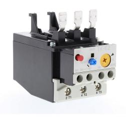
Fuji Electric TK-E2 series thermal overload relay, 12.0-18.0A adjustable, bi-metallic, direct mount power connection(s). For use with SC-E1x, SC-E2x and SC-E2Sx contactors.
