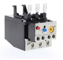
Fuji Electric TK-E2 series thermal overload relay, 9.0-13.0A adjustable, bi-metallic, direct mount power connection(s). For use with SC-E1x, SC-E2x and SC-E2Sx contactors.
